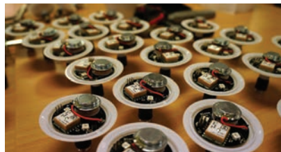
Featuring around 1,000 light bulbs, Bloom was on display at Canary Wharf (top). Inside each bulb is equipped with Wi-Fi, GPS and IoT intelligence which makes it location-aware.
