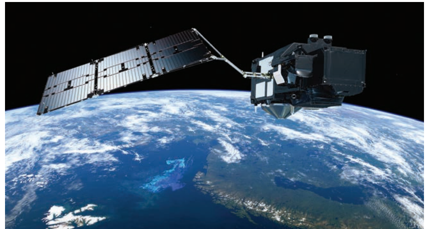
The ESA's Copernicus mission is based on two identical satellites – Sentinel-2A and Sentinel-2B – which cover all land surfaces, large islands, inland and coastal waters every five days. Working in unison, the two satellites optimise global coverage and data delivery for numerous applications.
