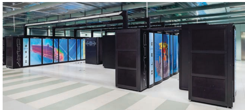
HLRS’ current supercomputer “Hazel Hen” is based on a Cray XC40 system and offers peak performance of 7.42 petaflops.
