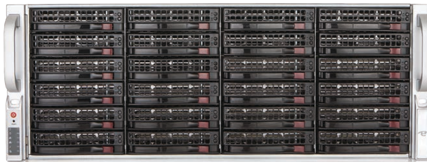
Endace said its 9200 Series can record more than a petabyte of network traffic at a sustained 40Gbps.
