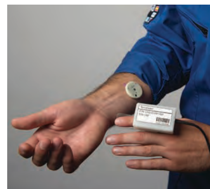
The Blood Pulse Wave sensor is a tonometer that will be used to record how the astronaut's arteries react to weightlessness. © ESA/NASA
